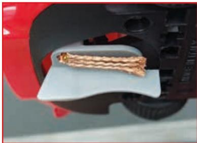
The guide blade on the Thunderslot cars are a unique shape which have been designed to cause minimal drag in the slot.
