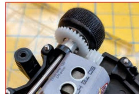
The motor is their own branded S-can called the Mach 21, the advertised max rpm is 21,500k. The narrow spur gear causes minimum drag against the nylon pinion giving you a silky smooth mesh.
