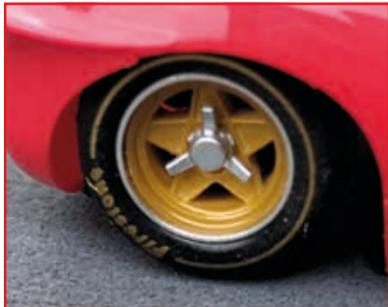
The five spokes, while inserts, are a fair representation and could be used to adapt a P3/P4 body to fit a Thunderslot chassis. They use alloy set screw hubs on the rear with push on lightweight plastic ones on the front.
