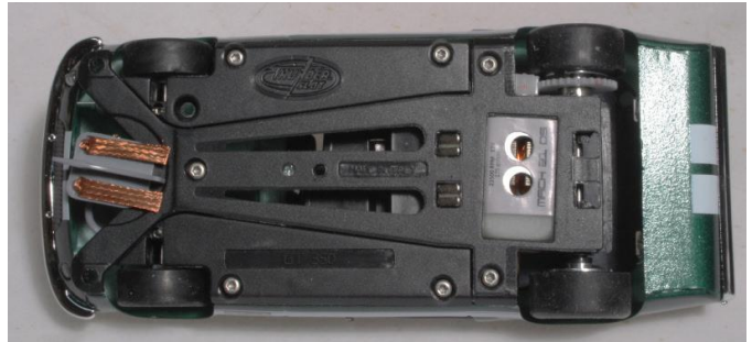
The front corners of the "pod" extend to the extreme front corners of the body---they are designed to serve as "skates" to limit the amount the model can roll or tilt in a corner.
