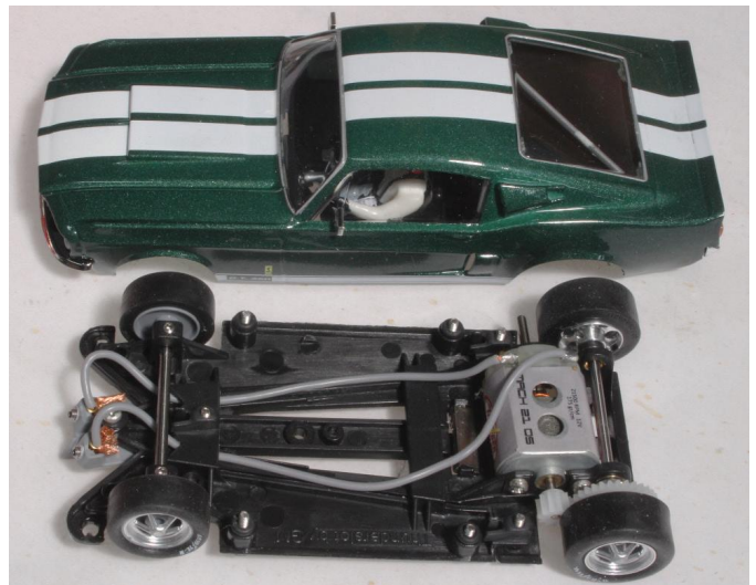
The S-Can motor is mounted as a sidewinder on the triangular pod that forms most of the chassis, extending forward to include the pickup.
