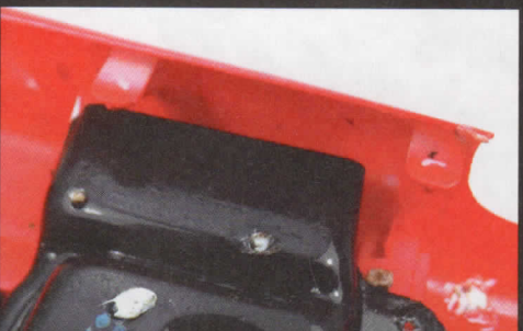
Tabs moulded to the bodyshell side for height adjustment
