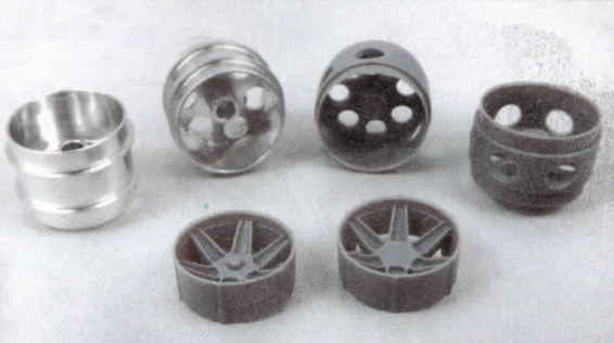
Very lightweight wheels. Note different inserts, one has a peg for locating the knock-off spinner
