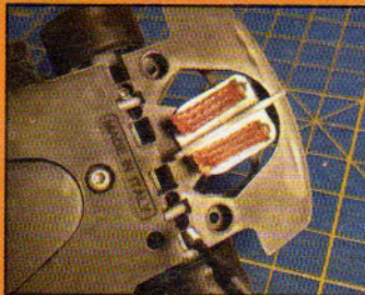
This done by placing the supplied grub screws in the holes at the front of the chassis - as shown here. You want the front wheels to barely touch the set-up plate for the ideal axle height.
