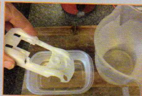
I am sure some of you have your own technique in straightening out twisted plastic bodies, but this is how I do it. The small tub below the shell contains boiling hot water, while the jug to the right is full of near ice-cold water. Place the shell into the boiling water for around 20 seconds, then twisting the shell into the correct position drop it straight into the cold water - repeat if necessary.
