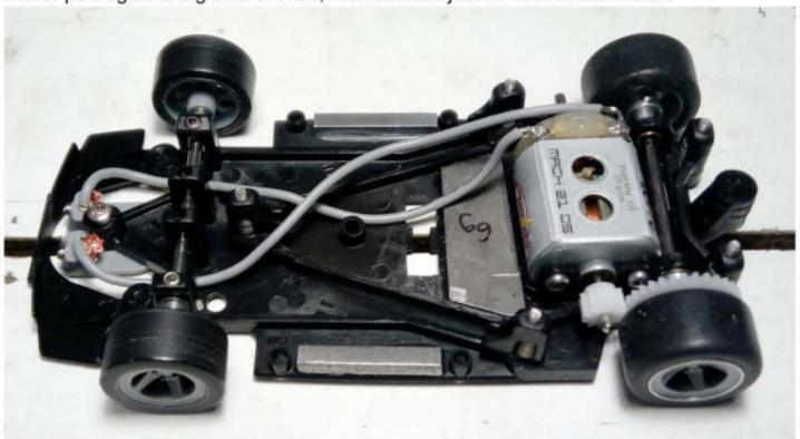
This piece of lead should weigh 6-8 grams and gets cut to fit that area of the pod. I normally have 8 grams in this position in front of the motor but for this car I am going to try 6 grams and see how stable it will be, I can always add more if needed. The way I cut the lead is to have a sharp blade from a box cutter that gets hammered into the top of and then through the lead the same way as a guillotine works, a few gentle blows does the job.
