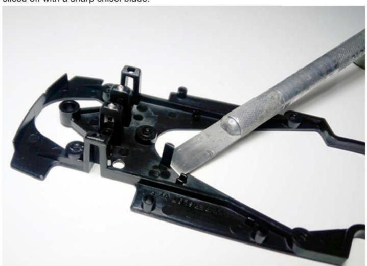
The spike is removed so that the lead wires don't catch on it and removing the words allows for better adhesion of the lead when glued to the sides of the outer part of the
