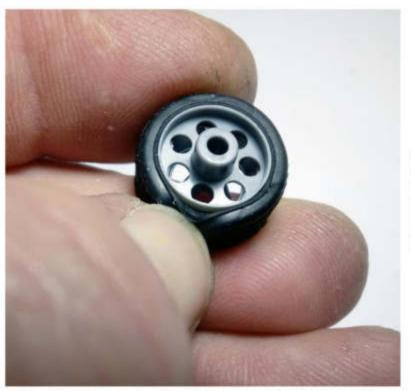
Fit the tires and then glue them to the rims - pic 15, open the tire a tad and apply the glue much like the rear tires, the cheap super glue is fine with the front tires.
