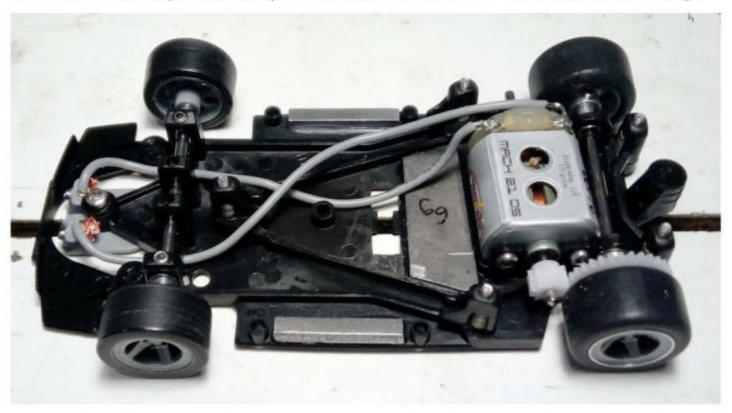
approximately 2.5 to 3 grams each side. Another piece of 1.5mm lead gets fitted under the rear axle where the magnet can go, it too should be 2.5 grams.
