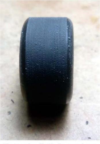
the car to bounce, making the car shudder while cornering. To trim the curve I use a plain old nail sanding stick. Like any sanding device, it leaves the curved edge rough but that is polished out with a soft cloth and turps.
