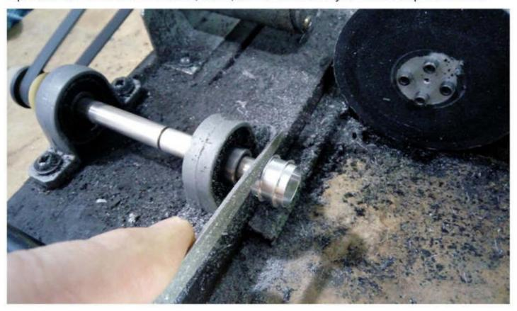
Spin the rims and scratch the area where the tyres sits with a file or sanding board to make the surface a little rough, enough to lose the polished surface, this gives the glue something to bite onto and hopefully it will grip better than on a smooth alloy surface - pic 7, wash away any dust before fitting the tire to the rim.
