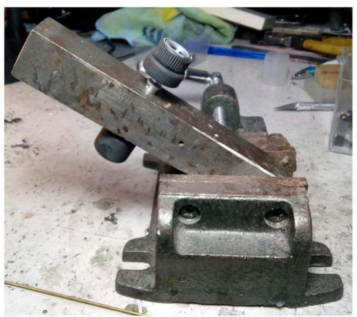
This tool comes in handy as it allows one hand to spin the rim while the other hands applies the glue. The block can be made from a square piece of wood or plastic or even an old chassis can be used.
