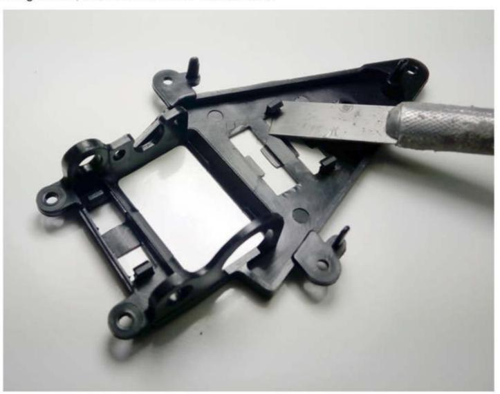
The areas where you remove plastic should be as flat and smooth as possible, no bumps is best to allow the glue to hold the lead properly.
