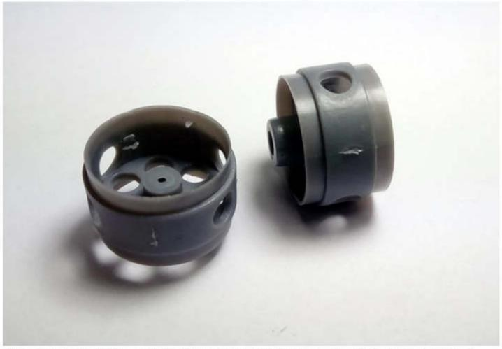
Sometimes the flash can be in the way enough to cause the rim to become out of round once the insert is fitted, best to remove the flash so the insert will fit without distorting the rim.
