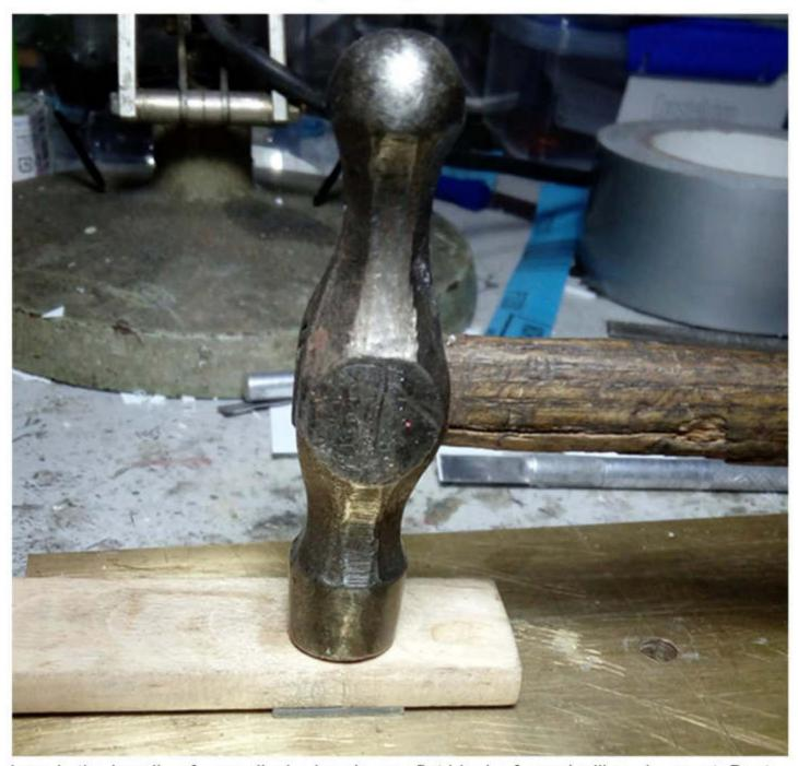
here is the handle of a small wire brush, any flat block of wood will works great. Best to also scratch the surface of the lead so it becomes clean and shiny, this is to remove any oxidation so the glue bonds to the clean lead and not the oxidised surface. The clean surface helps for a better bond making it less likely for the lead to become loose during racing.
