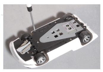
The set-screws for the wheels and gear, for the pod and the body-mounting screws are not the usual Phillips head or Allen hex but Torx T6. There are two holes for Torx Allen screws on each side of the chassis that can be turned in or out to adjust the height of the body on the chassis. The front wheels are plastic. The rear wheels are set-screw-mount aluminum with two-piece tires that have a foam inner strip to provide a claimed "air" suspension.
